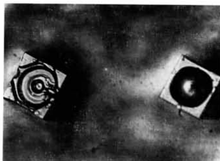
Fig. 6. Hillocks produced by thermal etching at 765–785°C ( \times 264 ).
