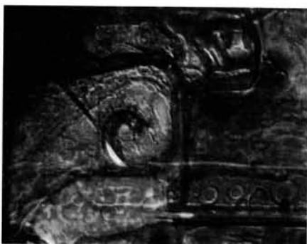
Fig. 8. Anticlockwise spiral on top of a whisker ( \times 510 ).
